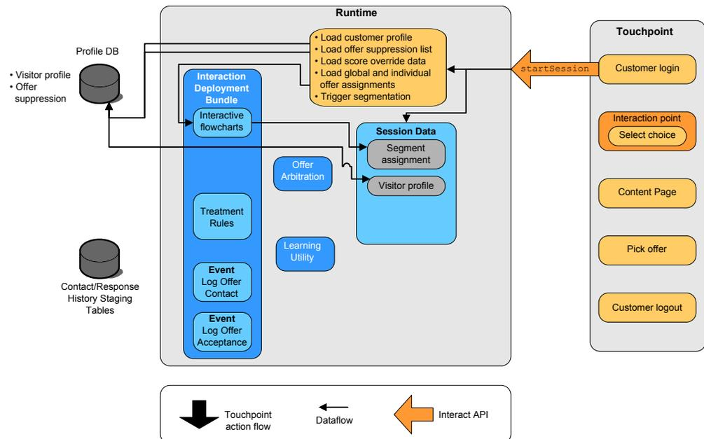
In this example, the `startSession` method does four things. First, it creates a new runtime session. Second, it sends a request to load the customer profile data into the session. Third, it sends a request to use the profile data and start an interactive flowchart to place the customer into segments. This flowchart run is asynchronous.
