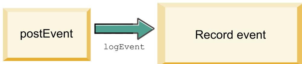
The `logEvent` method is called by the runtime server whenever the Interact API posts an event that is configured to log as a contact or response. Use this method to log contact and response data to a database or file for reporting and learning purposes. For example, if you want to algorithmically determine the likelihood of a customer accepting an offer based on criteria, use this method to log the data.
