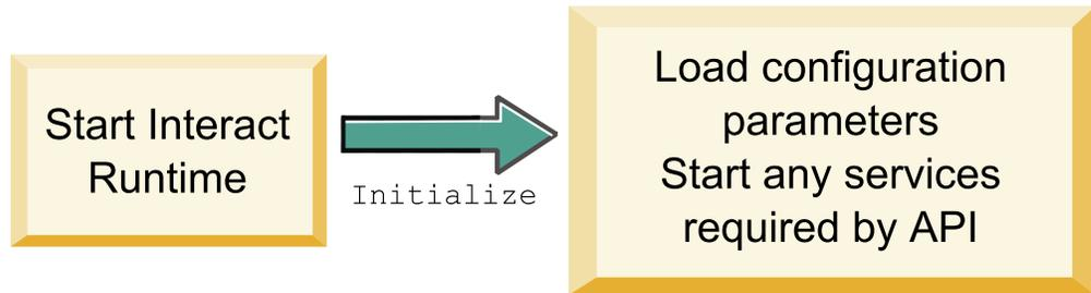
The initialize method is called once when the runtime server starts. If there are any operations that do not need to be repeated, but may impede performance during runtime, such as loading static data from a database table, they should be performed by this method.
