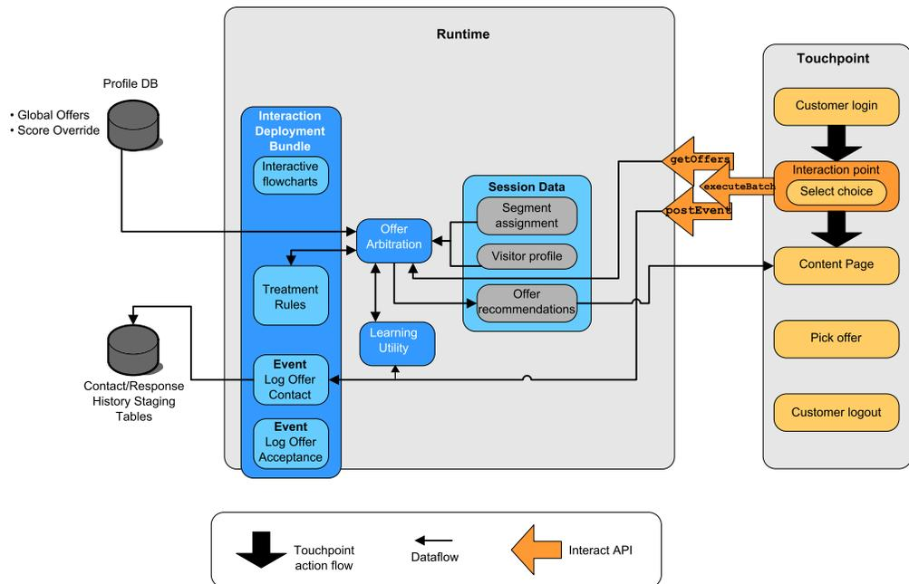
The executeBatch method enables you to call more than one method in a single call to the runtime server. This particular executeBatch calls two other methods, getOffers and postEvent. The getOffers method requests a list of offers. The runtime uses the segmentation data, the offer suppression list, the treatment rules, and the learning module to propose a set of offers. The runtime returns a set of offers which are displayed on the content page.
