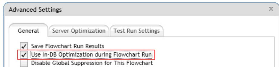
When you save and run the flowchart, in-database processing will be used whenever possible, if you are using in-database optimization.
