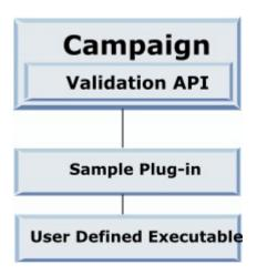
The executable may be written in any language, but must reside on the Unica Campaign server and be executed on the server. The plug-in that calls the executable sends in an XML file that contains the information to be validated; for example, the user editing the object and the before and after values for all standard and extended attributes of that object. Unica Campaign expects results information in the form of an XML file in return.
